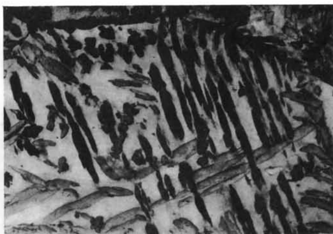
Fig. 5. Initial alloy. Etched with ammoniacal hydrogen peroxide. \times 150 .
