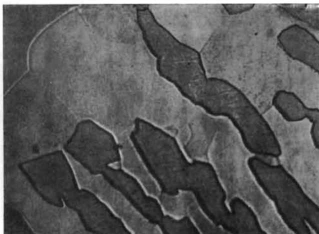
Fig. 7. Alloy annealed 13 hr. at 500^{\circ}\text{C} . Electro-polished and etched by method (B) followed by method (C). \times 1200 .
