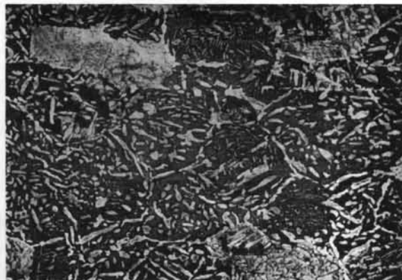
Fig. 3. Alloy annealed 13 hr. at 500^{\circ}\text{C} . Etched with aqueous acid ferric chloride. \times 25 .
